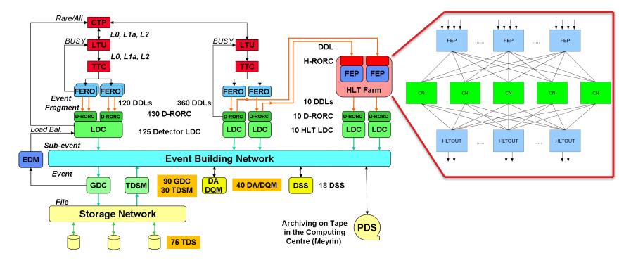
Different technologies/techniques used in DAQ/HLT e.g. Ethernet <-> Infiniband
