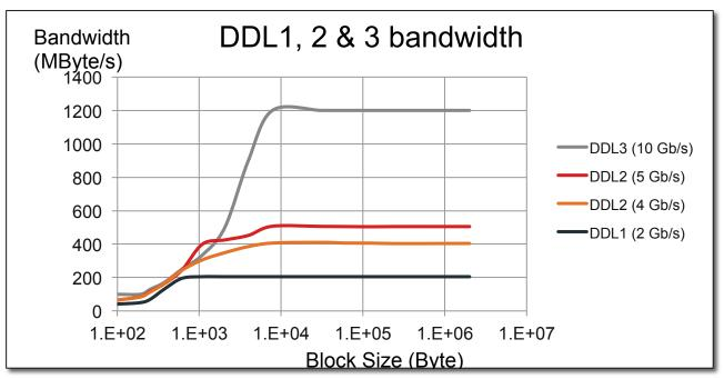
DDL2 at 4 and 5 Gb/s (according to needs) ready for Run 2
