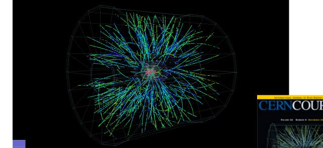
Full GPU tracking available in the HLT since Pb+Pb 2011; based on CA algorithm
