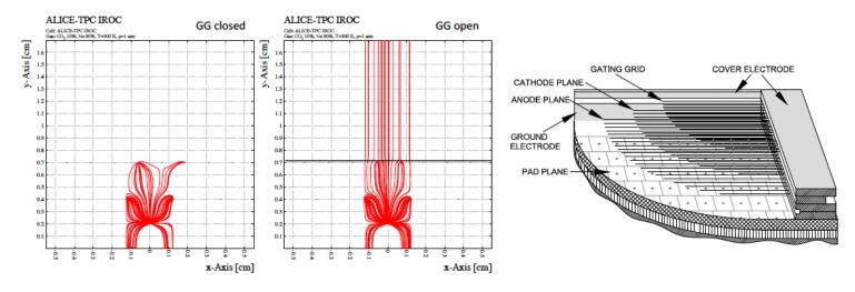
Ions from the amplification region require finite drift time to reach the gating grid With current ALICE TPC gas: ~100 μs drift + 180 ~μs gating grid closing time **Rate limited to ~3.5 kHz**
