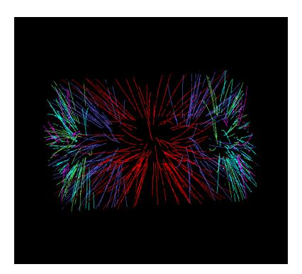
Operated in continuous mode: self triggered electronic At 50kHz: on average 5 events in TPC drift time of ~100 µs -> Factor 5 in data volume for online systems to read-out and process
