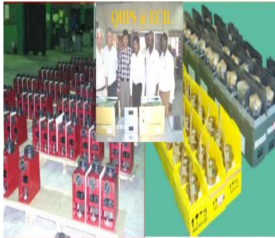
Precision Magnet Positioning System (PMPS) Jacks
