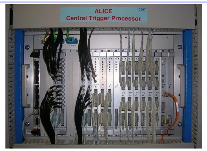
CTP triggers are sent to Local Trigger Units (LTUs) where conversion to output format occurs
