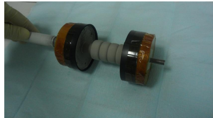
Au coated structure with a 4 mm thick Nickel coating Bruno Spataro, INFN Frascati
