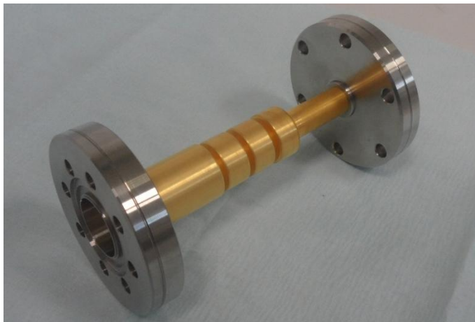
Fitting test between mandrel and CF flanges
