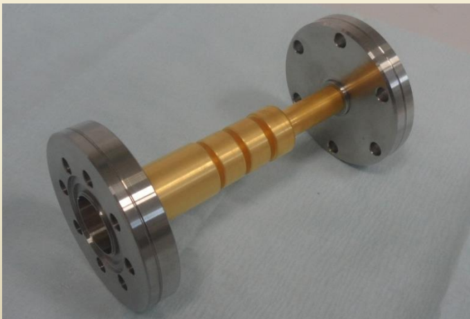
Fitting test between mandrel and CF flanges
