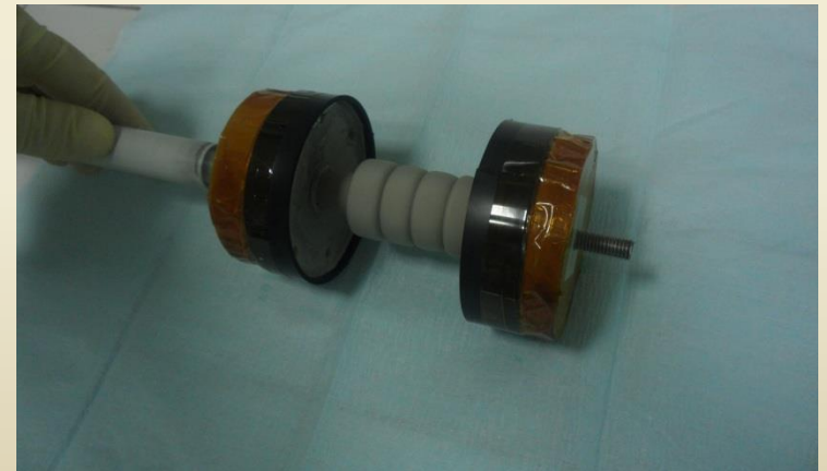
Au coated structure with a 4 mm thick Nickel coating
