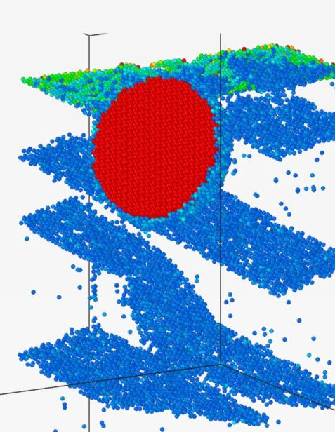
Extensive stacking faults are observed in the presence of large Fe precipitates close to the surface. A depression tends to form on the surface, creating a Cu-Fevacuum interface and facilitating atom evaporation.
