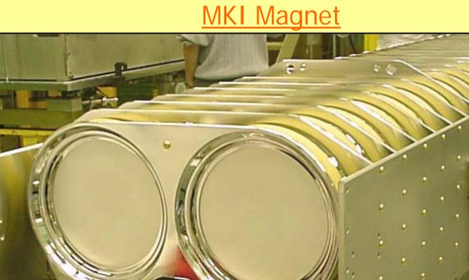
The travelling wave kicker magnet yoke is made of ferrite cores. Screen conductors mounted in a ceramic tube (lower left of figure), are placed in the aperture of the magnet: these conductors provide a path for the image current of the, high intensity, LHC beam and screen the ferrite against wake fields.
