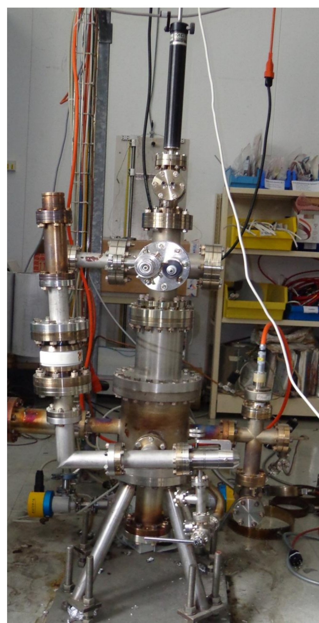
DC-spark system at CERN
