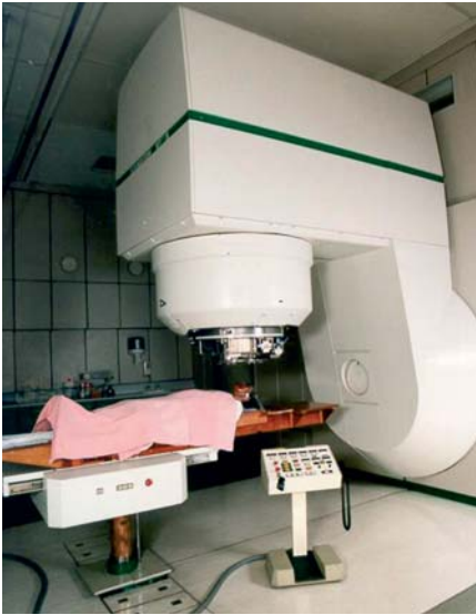
Figure 3. The neutron therapy gantry of the National Acceleration Center (Faure, South Africa) uses the p+Be reaction with 66 MeV protons.
