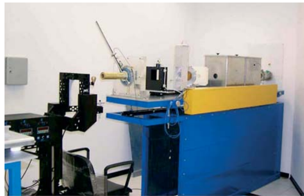
Figure 17. The CATANA set-up to treat eye tumours and malformations ( www.lns.infn.it/CATANA ).
