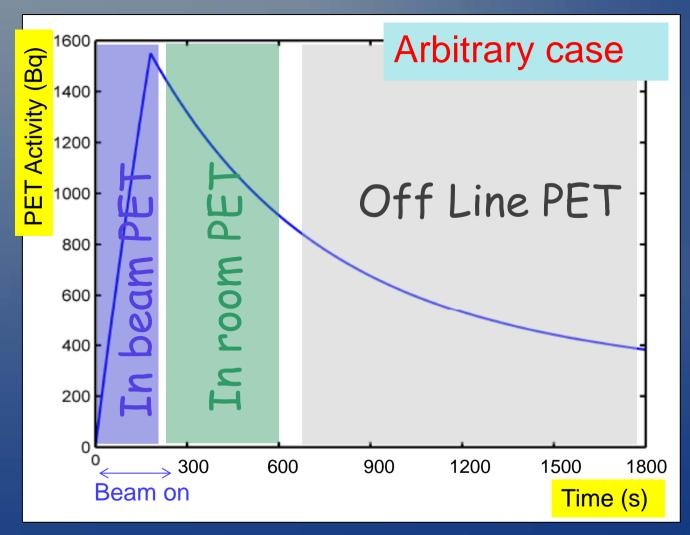
Detector acceptance should be such to collect enough statistics in the beamon time
