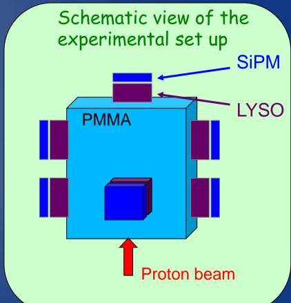
The LYSO crystals in contact with PMMA phantom  $(5 \times 5 \times 7 \text{ cm}^3)$
