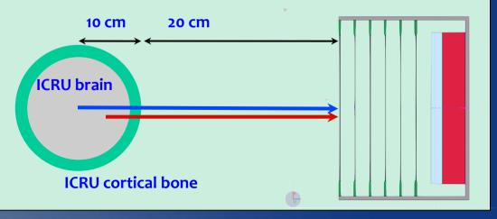
FLUKA sim. of tracker made of 6 planes of 500  $\mu m$  XY sci fi
