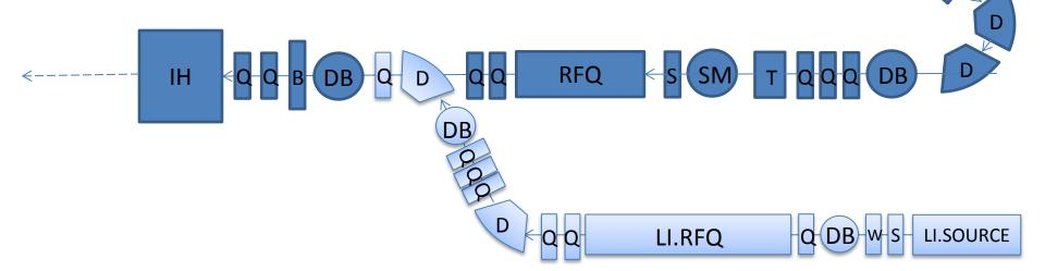
**Legend:** B - Buncher, D - Dipole, DB - Diagnostic Box, IH - Interdigital H accelerating structure, Q - Quadrupole, RFQ - Radio Frequency Quadrupole, S - Solenoid, SM - Steering Magnets, T - Beam transformer, W - Wien Filter
