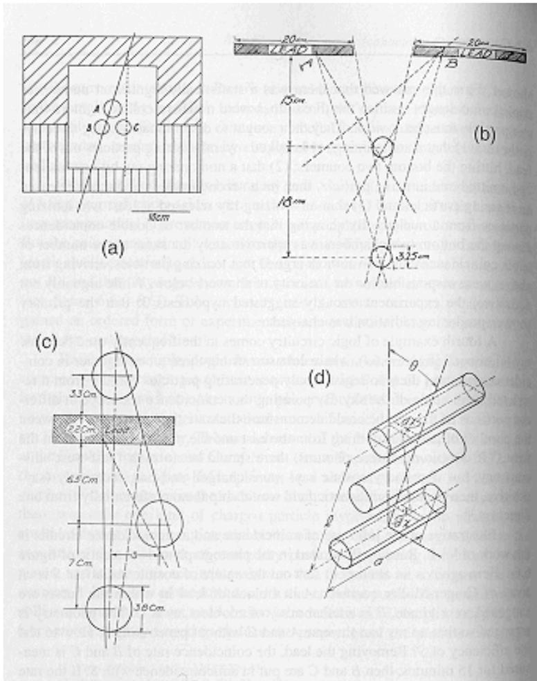
By performing coincidences of Geiger Müller tubes e.g. the angular distribution of cosmic ray particles could be measured.
