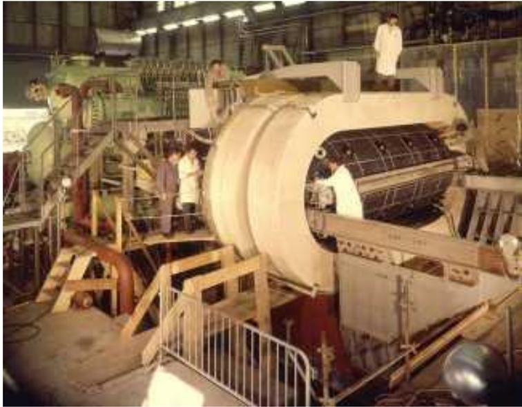
Gargamelle, a very large heavy-liquid (freon) chamber constructed at Ecole Polytechnique in Paris, came to CERN in 1970. It was 2 m in diameter, 4 m long and filled with Freon at 20 atm.
