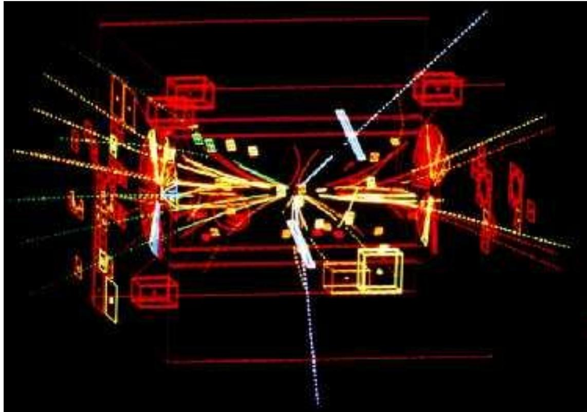
This computer reconstruction shows the tracks of charged particles from the proton-antiproton collision. The two white tracks reveal the Z's decay. They are the tracks of a high-energy electron and positron.
