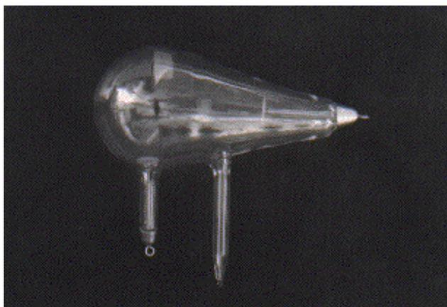
This tube is a glass bulb with positive and negative electrodes, evacuated of air, which displays a fluorescent glow when a high voltage current is passed through it. When he shielded the tube with heavy black cardboard, he found that a greenish fluorescent light could be seen from a platinum screen 9 feet away.
