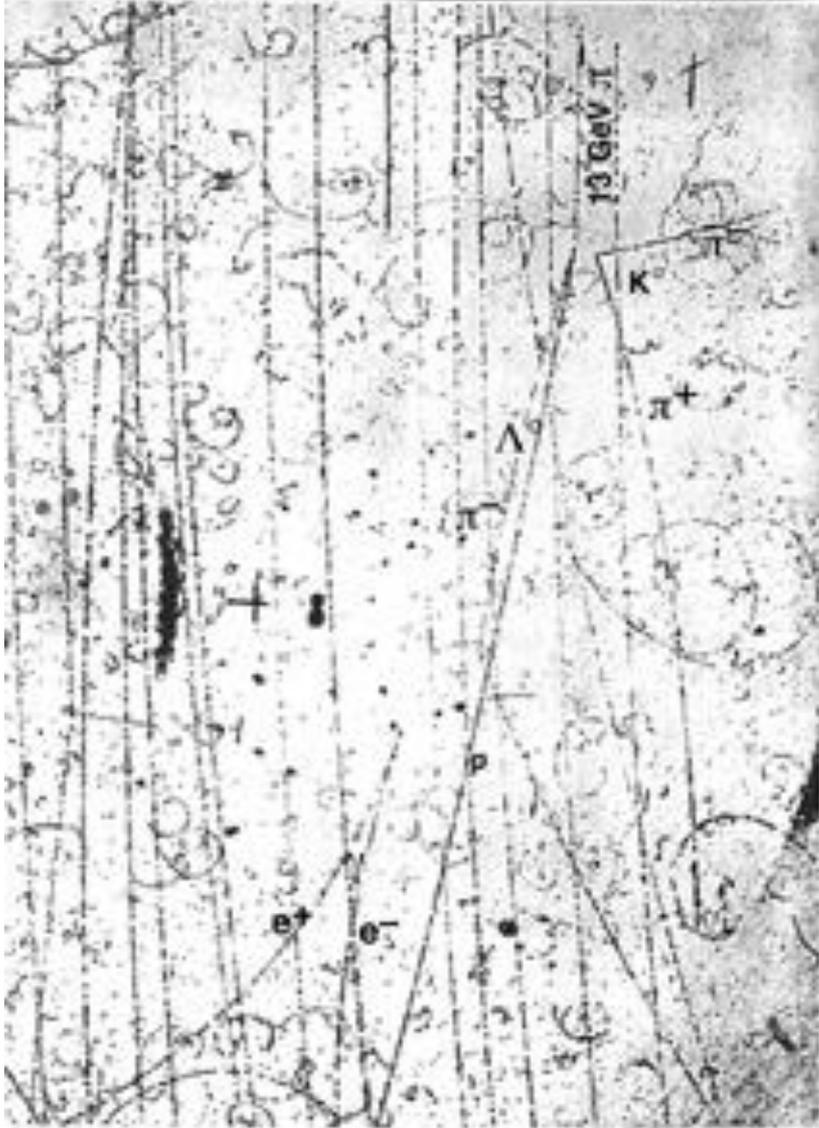
In the bubble chamber, with a density about 1000 times larger than the cloud chamber, the liquid acts as the target and the detecting medium.
