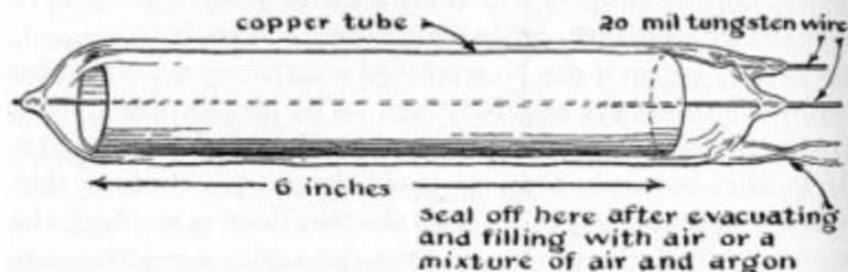
Fig. 9. Typical construction of a copper-in-glass counter. Following this general design, counters have been made from 0.5 cm to 10 cm in diameter.
