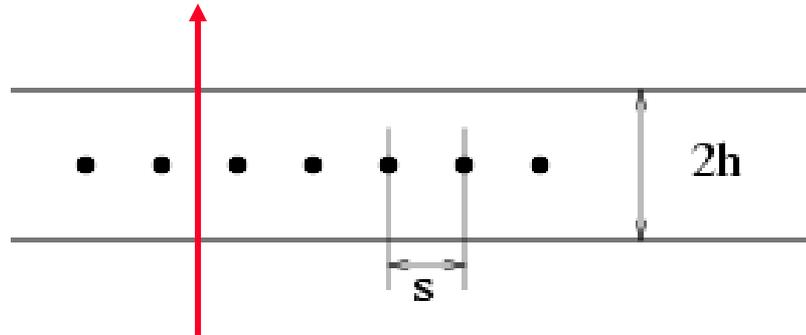
Measuring this drift time, i.e. the time between passage of the particle and the arrival time of the electrons at the wires, made this detector a precision positioning device.
