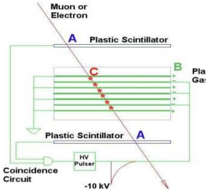
A charged particle traverses the detector and leaves an ionization trail.
