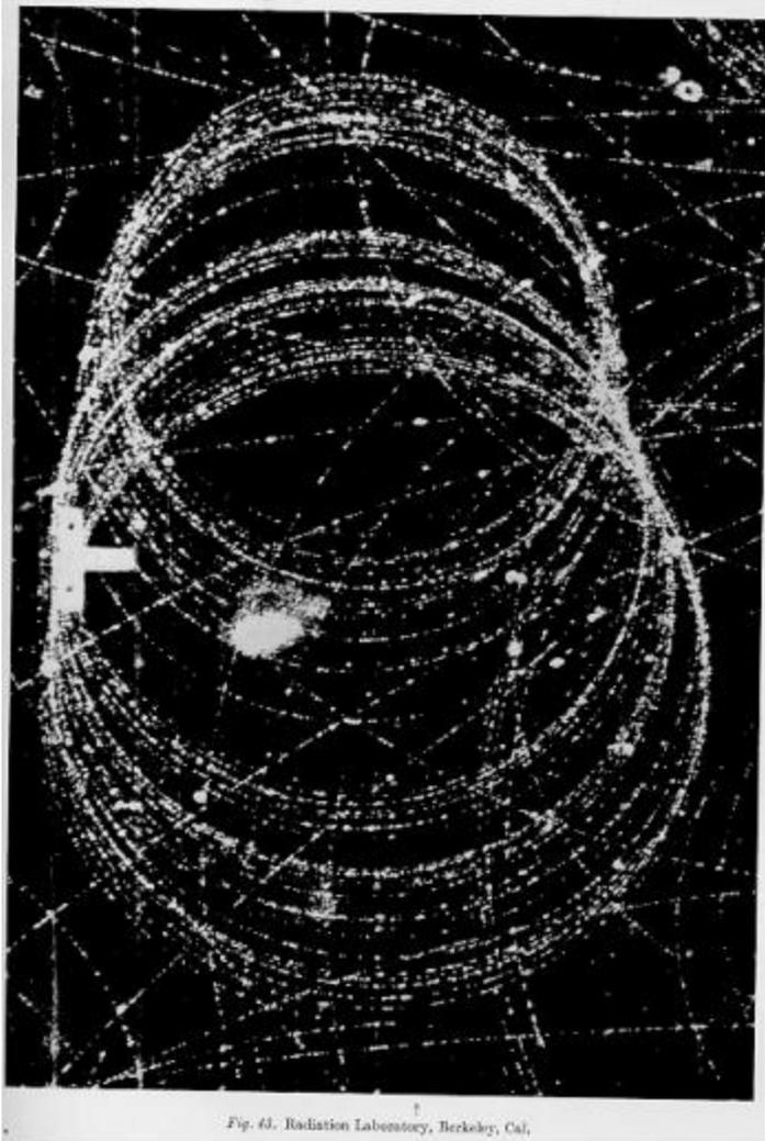
The picture shows an electron with 16.9 MeV initial energy. It spirals about 36 times in the magnetic field.
