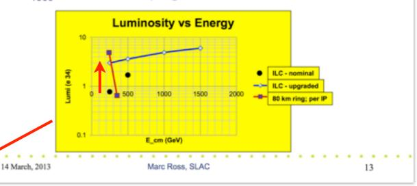
x4 upgrade @250GeV Snowmass  $e^+e^-$  Collider Luminosity (fb<sup>-1</sup>) based on  $3\times10^7$  s running time for ILC & LEP3/TLEP
