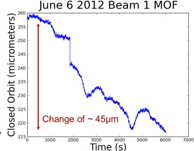
A closed orbit shift of 45 µm corresponds to a Q' shift of 0.8 units. A 40% change!
