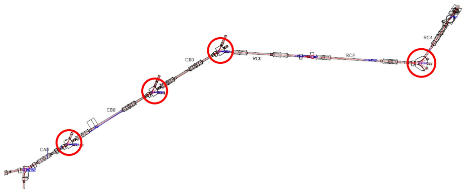
Figure : The kickers and switchyards.
