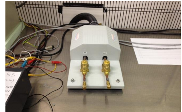
Inlet/outlet pipes for test section
