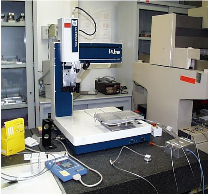
I&J Fisnar 750 gluing robot dispensing
