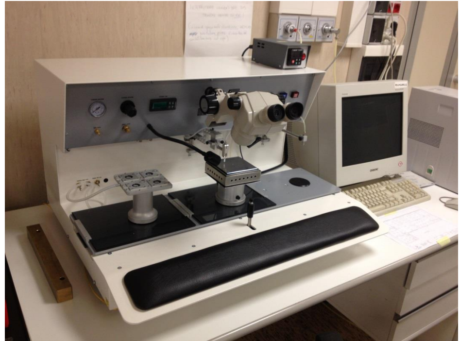
Die-attach machine Cammax DB 600
