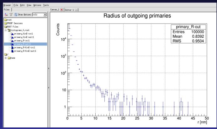
It registers the distance-to-axis and kinetic energy distributions at the entrance and exit of the scoring cylinder
