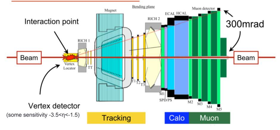
Fully instrumented within  $1.9 \le \eta \le 4.9$ Trigger:  $p_{\mu} > 3$  GeV,  $pt_{\mu} > 0.4$  GeV,  $m_{\mu\mu} > 2.5$  GeV
