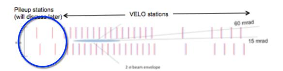
Silicon sensors at 8.2<R<42mm and z>-315mm 40 MHz readout Very effective VETO
