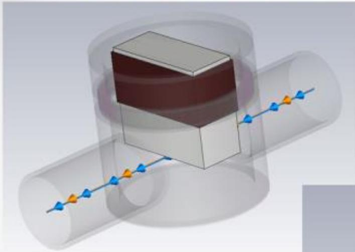
The main problem is the vacuum cavity between the RP and the flange: box RP and cylindrical flange.
