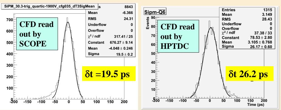
QUARTIC and SiPM signals amplified, sent to CFD, then to scope, calculate  $\Delta t$ (SiPM-Qi) and average over 6 bars. Repeat for HPTDC readout. Difference between the measurements is dominated by 16 to 18 ps resolution of SiPM HPTDC
