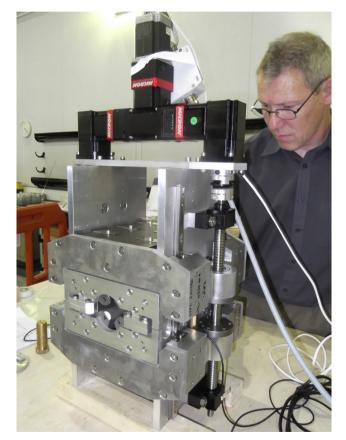
CLIC drive beam PM quadrupole prototype. ASTeC and Technology in collaboration with CERN
