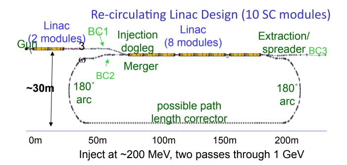
Concept and design of SCRF based linac capable of operating at 1 MHz (stage II)
