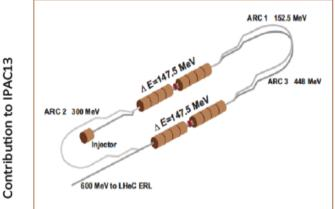
Figure 2: Consequent upgrade to LHeC pre-accelerator. By modifying the machine backleg to include a second full cryomodule, the recirculator can deliver higher beam energy of 600 MeV.
