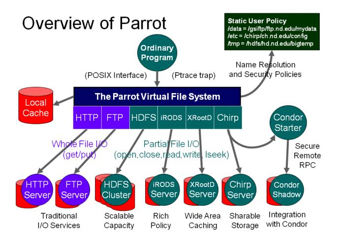
Parrot is a transparent user-level virtual filesystem that allows any ordinary program to be attached to many different remote storage systems, including HDFS, iRODS, Chirp, and FTP + CVMFS
