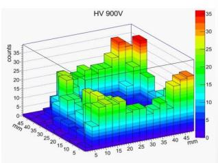
• Triple GEM with Boron converter for slow neutrons in position 2
