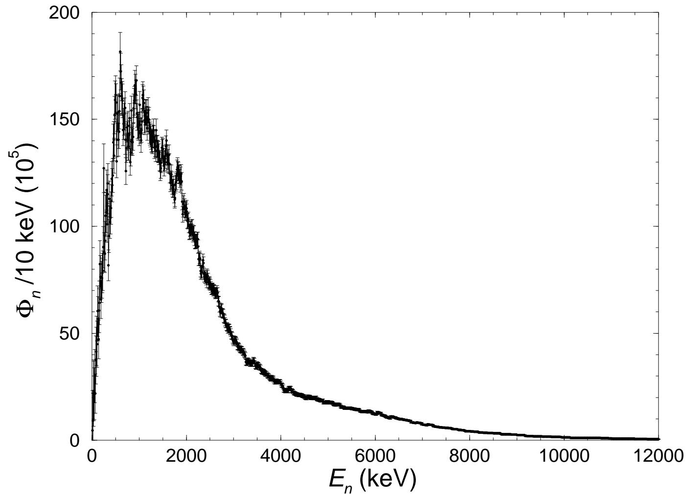
Neutron fluence measured by means of a fission chamber of PTB Braunschweig
