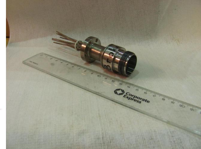
HV feedthrough was broken
