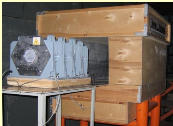
Lead target + uranium blanket
