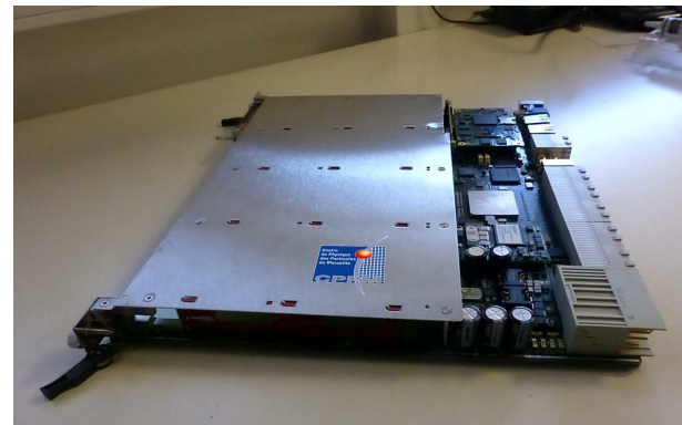
ATCA board with 4 AMC mezzanines
