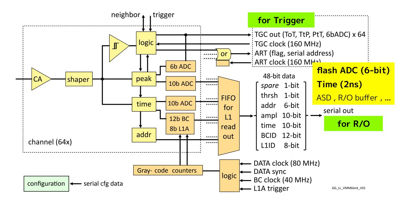
64ch. per chip , 512mW/ch. , ~40k chips
