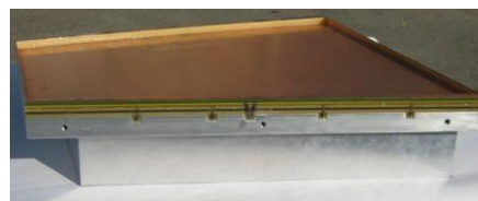
ALICE triple GEM TPC end-cap module
