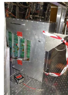
ALICE triple GEM TPC end-cap module
