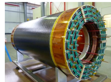
KLOE2 inner tracker: 4 layers of triple cylindrical GEM detectors
