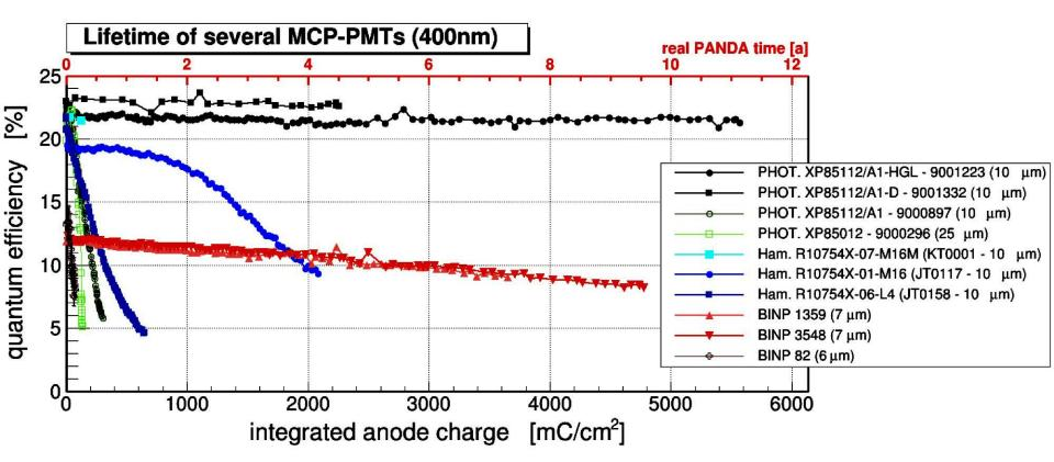
Dependence of the Quantum Efficiency on the Integrated Anode Charge for a variety of MCP-PMT sensors measured by PANDA collaboration. The performance of the ALD treated samples from Photonis USA is shown by the top curves.
