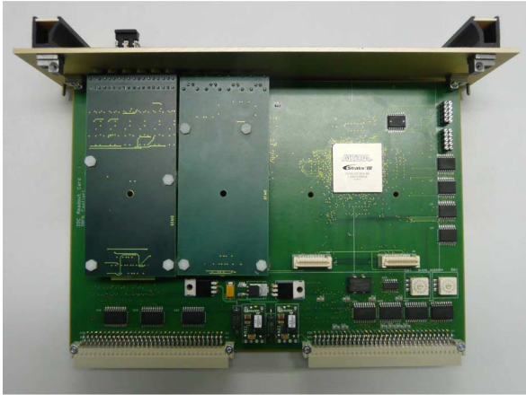
Fig. 5. The ZDC Readout Card (ZRC). It is a custom board with an Altera Stratix III FPGA.
