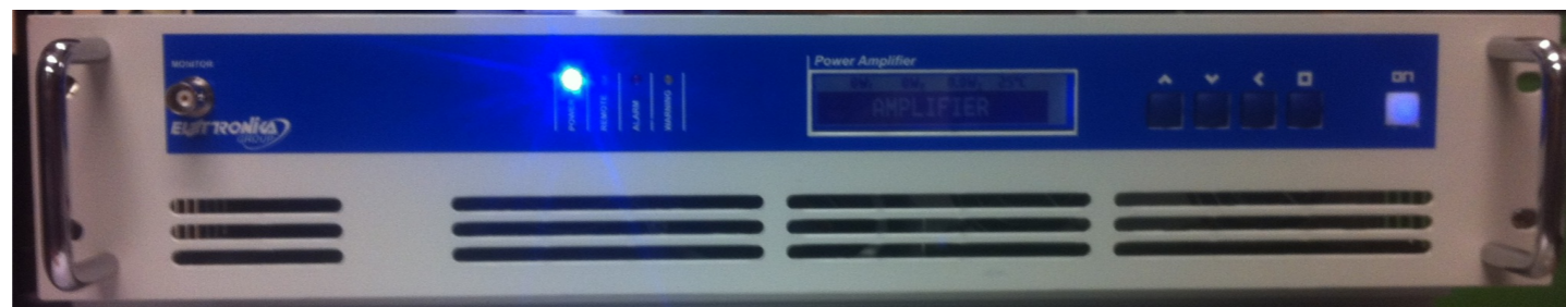
Prototype 100 MHz, 750 W solid state amplifier for SM18 test stand
