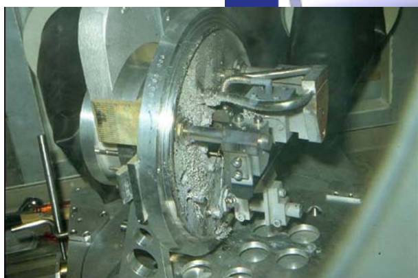
Liquid metal target: Cracked container welds
