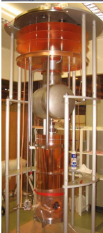
Nb/Cu cavity on its test frame
