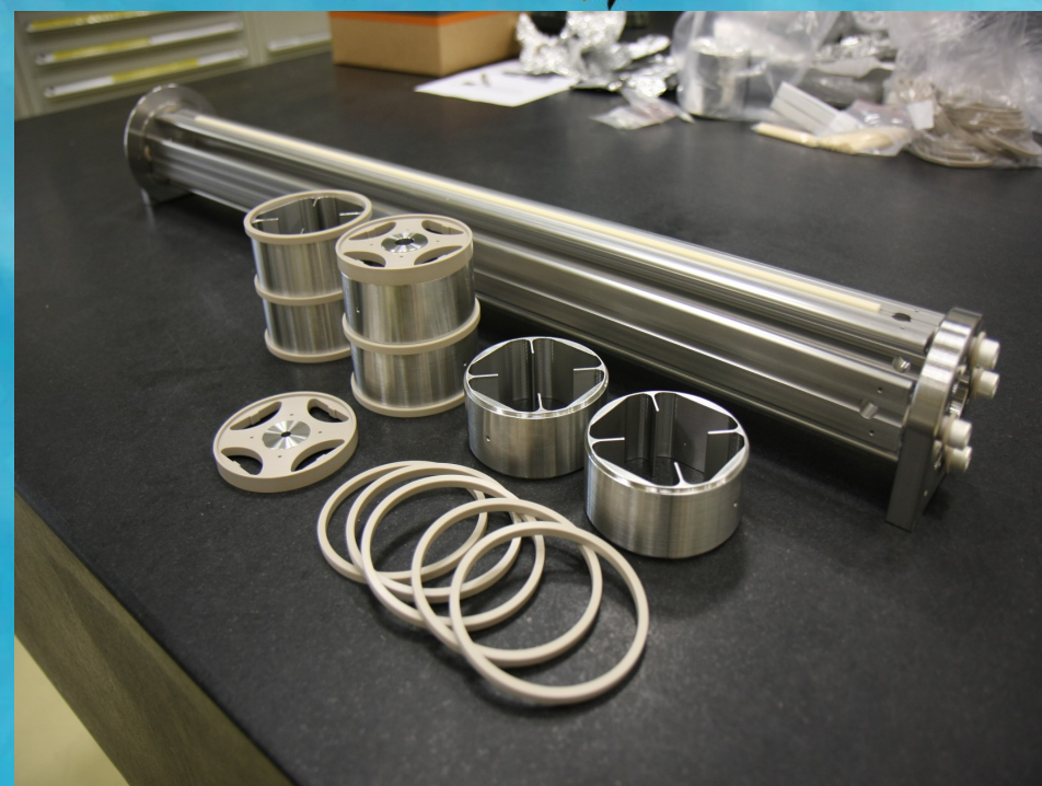
The new RFQCB is being built for the test stand
