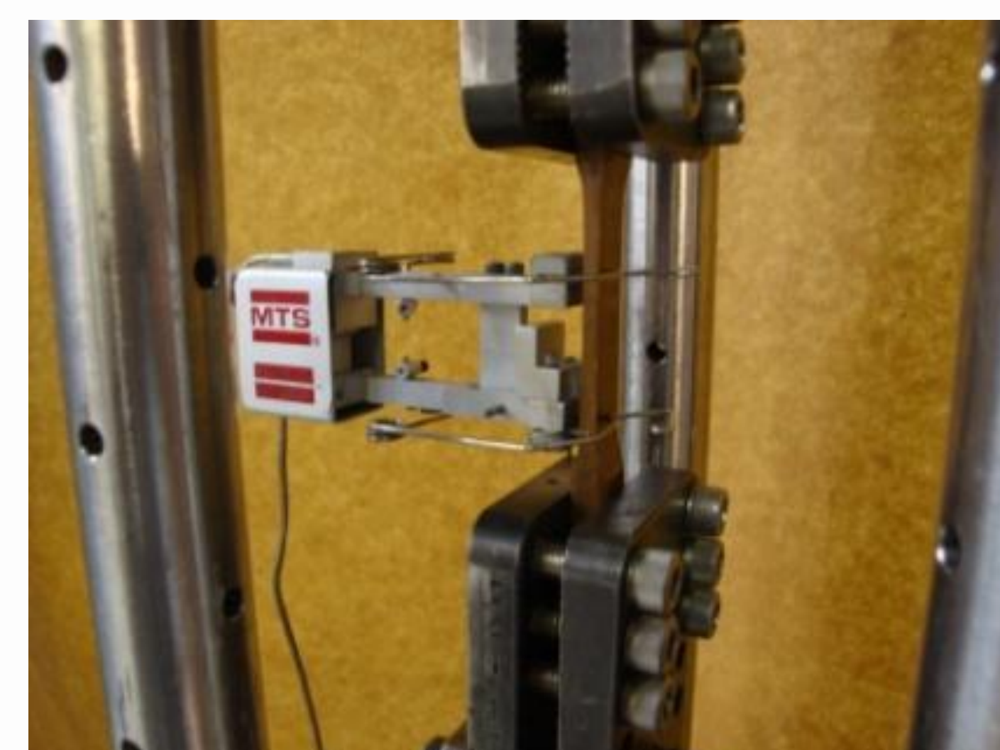
FIGURE 1. Tensile test setup
