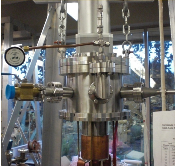
Cold Head of a cryocooler
