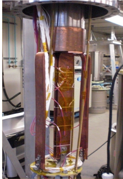
Conductive path for heat transfer
