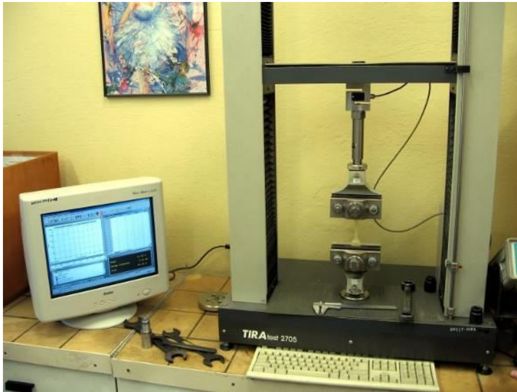
TIRAtest Table Unit 2705 and its upgrade with LN2 vessel
