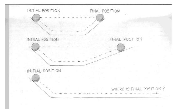
Conclusion: object will continue to move In a straight line with a steady speed.
