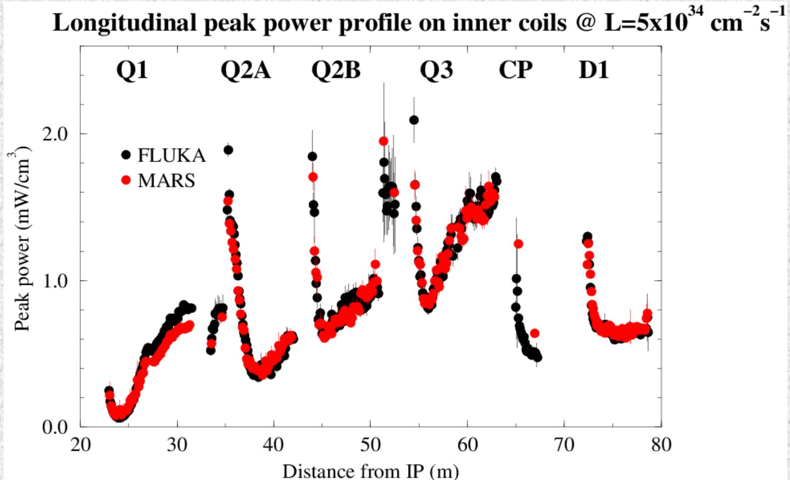
Peak power density is averaged over the **full cable width; 50 cm** beam screen interruption in the interconnects
