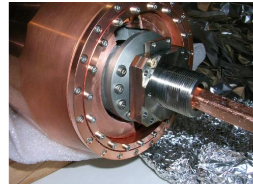
Oversize Outer Housing w/ Flats that prevent rotation in jaw supports
