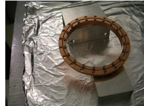
Trapped bearing in ring that is fixed to the collimator jaw
