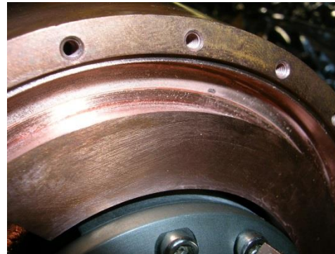
Close-up of ridge where bearing rolls
