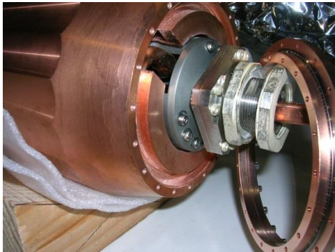
Attaching outer ring to collimator
