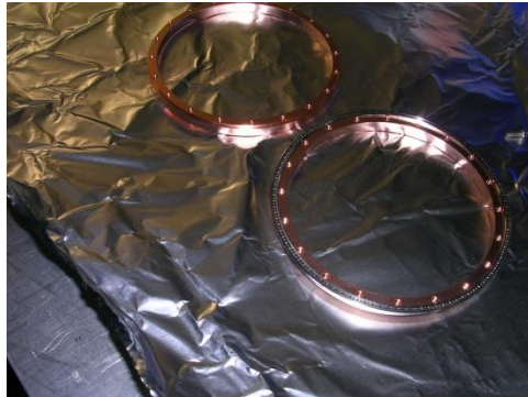
Ceramic bearing in race & the 2 rings that capture it
