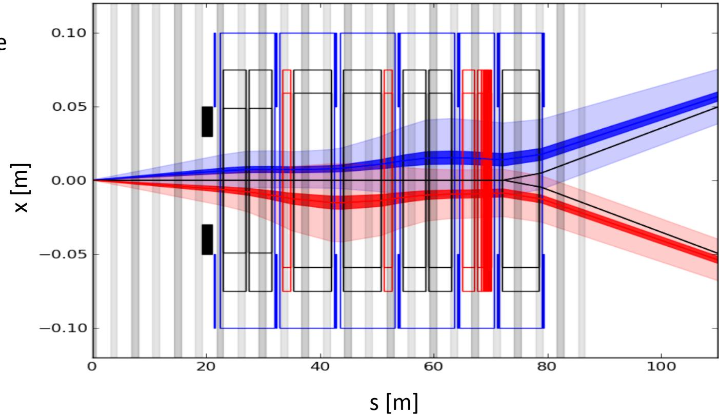
Smaller crossing angle and beam size in the crossing plane.
