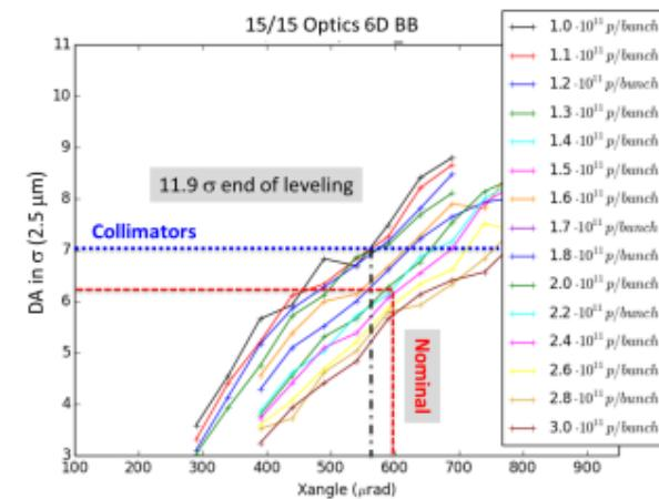
Beam beam effects (pacman, orbit, DA) and wire compensation under study.
