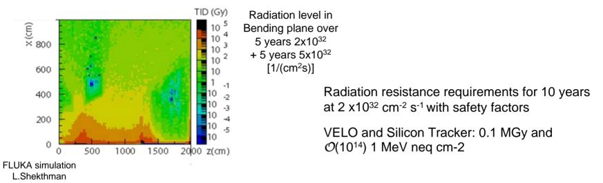
Machine induced background for beam1 from the tertiary collimators (V.Talanov) Lifetime 30h with nominal machine → Loss rate 3x10<sup>9</sup> p/s in IR7 (3x10<sup>6</sup> p/s on TCT) → 2 x 10<sup>6</sup> charged particles(h+µ)/s at LHCb cavern with currently installed shield.
