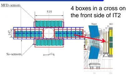
Main function: to monitor radiation load on Silicon Tracker sensors
