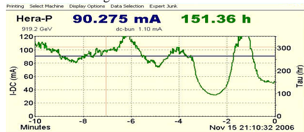
Figure 10: Beam lifetime measurement: Used mainly for "long term" measurements. For fast and efficient background tuning the significance was limited.
