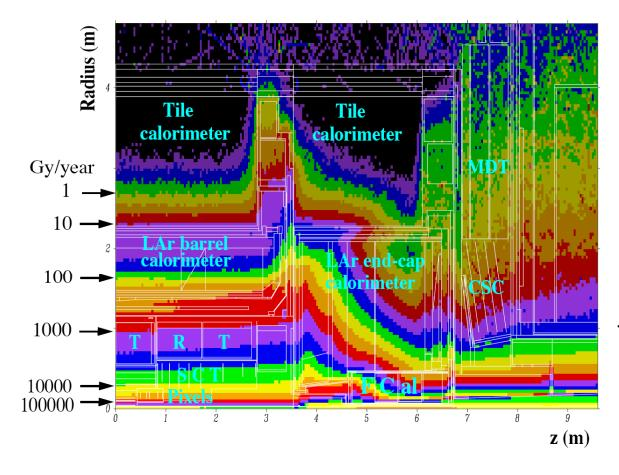
Total ionising dose per year  $(\mathcal{L} = 10^{34} \text{ cm}^{-2} \text{s}^{-1})$  calculated by GCALOR in one quarter of the central part of the detector. The locations of the inner detector sub-systems, of the different calorimeters and of the inner end-cap muon stations are indicated. The scale on the left gives the integrated dose per year corresponding to the various isolines.
