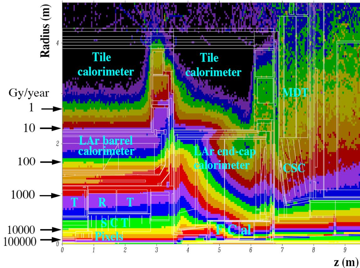
**Total ionising dose per year** ( $\mathcal{L} = 10^{34} \text{ cm}^{-2}\text{s}^{-1}$ ) calculated by GCALOR in one quarter of the central part of the detector. The locations of the inner detector sub-systems, of the different calorimeters and of the inner end-cap muon stations are indicated. The scale on the left gives the integrated dose per year corresponding to the various isolines.
