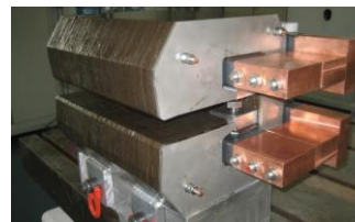
LHeC dipole with one-turn conductor & air cooled interleaved laminations [1 mm iron, 2 mm plastic] (CERN)
