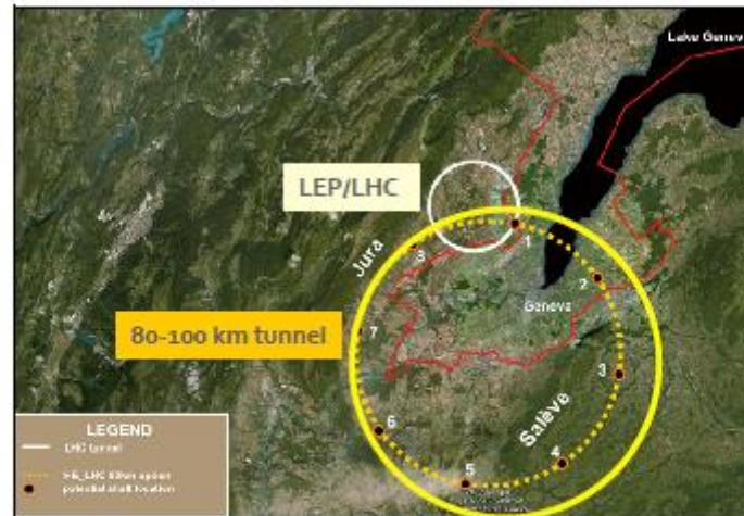
Fig. 2: A possible implementation of the 80 km tunnel (dashed circle) that would host TLEP and the VHE-LHC in the Geneva area, taken from Ref. [9]. The 100 km version (full line) is currently under study.
