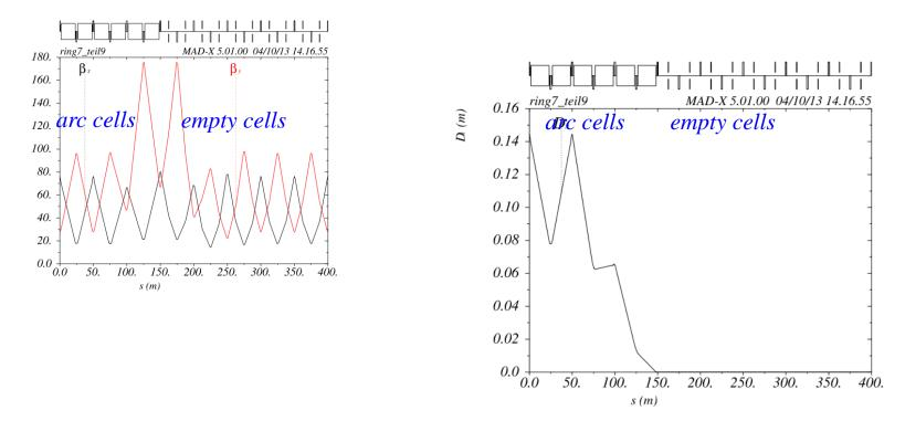
to be optimised:  $\beta_y$  at matching section, needs an additional quadrupole lens  $\rightarrow$  already built in but not used yet. and / or optimisation of the lens positions
