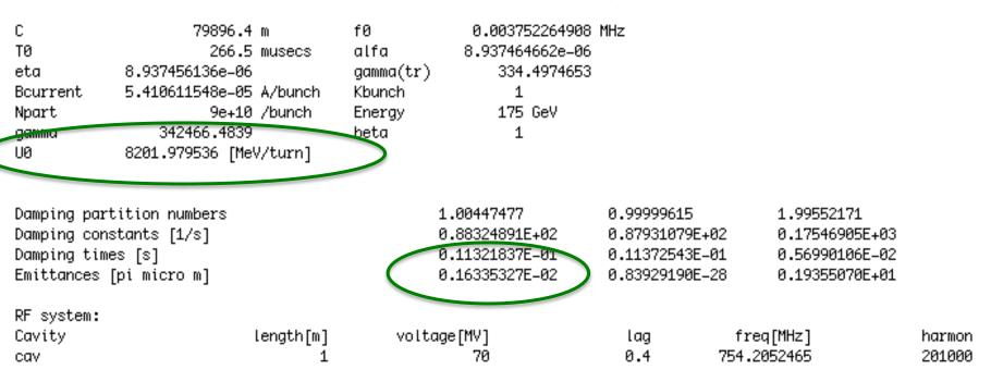
Nota bene: Emittance is as before nicely small .. still smaller than the design value (2nm). however for a theoretical, ideal lattice without coupling, beam-beam, solenoid fields, tolerances  $\rightarrow$  error tolerances to be considered,  $\rightarrow$  how realistic is 2nm and 1 permille for  $\varepsilon_v / \varepsilon_x$
