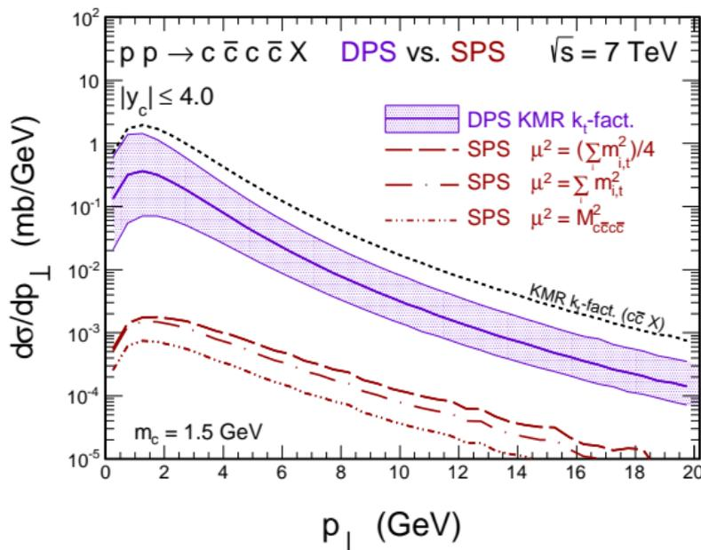
dependence on renormalization and factorization scale of SPS
