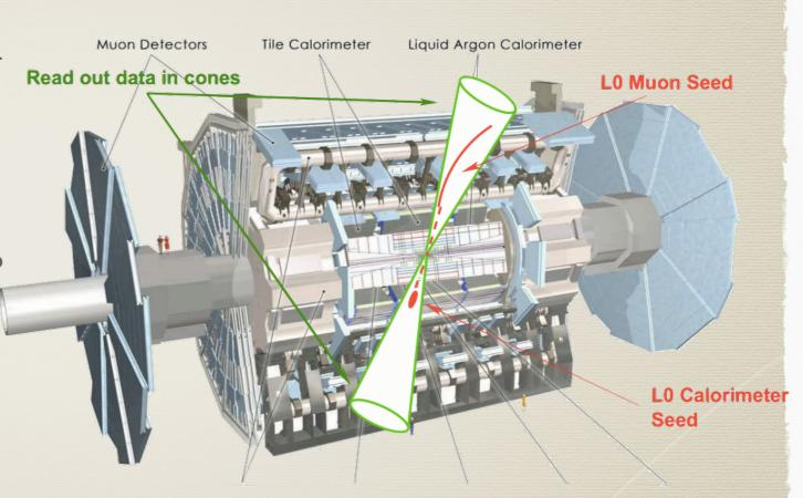
Toroid magnets Solenoid magnets SCT tracker Pixel detector TRT tracker
